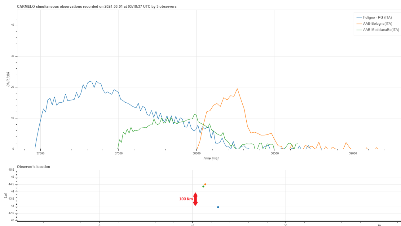
Figure 11 – Simultaneous reception from three observers: the waveforms are similar.
