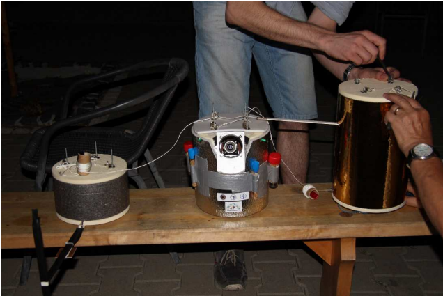
Figure 3 – Stratospheric balloon STRATO 02/2015 payload: cosmic ray particles detector (left); MeteorCam03 (middle); modules of JULO-X probe, transmitter for SkCube and Geiger-Müller tubes (right).
