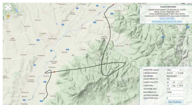
Figure 1 – Projected flight trajectory of stratospheric balloon STRATO 02/2015 to the Earth surface.
