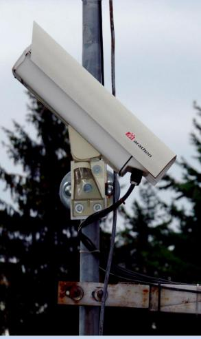
using spectra are recorded using spectrograph camera equipped with 1/3" CCD chip and holographic diffraction grating. The effective resolution of 720 x 576 px and density 500 lines / mm grating allow resolution of 3.04 nm / px in the range of 585 to 703 nm. The system is calibrated using a neon calibration lamp. The detection itself is performed using UFOAnalyzer software. The cameras on Valašské Meziříčí Observatory are employed in the CEMENT and EDMOND European meteor network.
